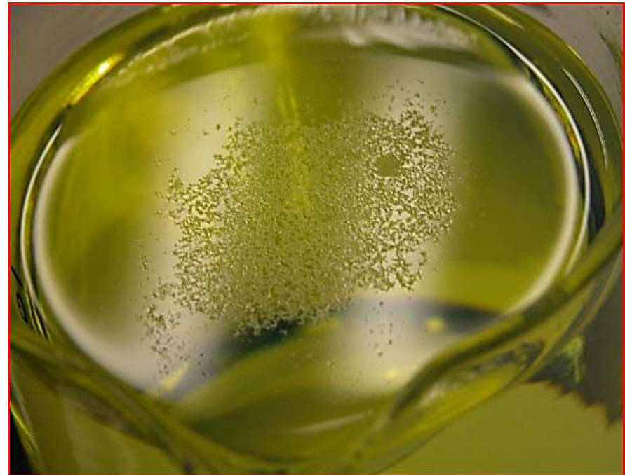
Two examples of B5 samples with a floating layer at the top.
