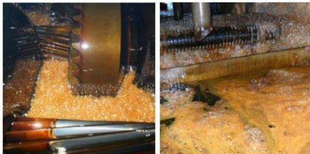
Pictures: lubricating oil foaming inside a machine during use and inadequate lubrication causing damage
