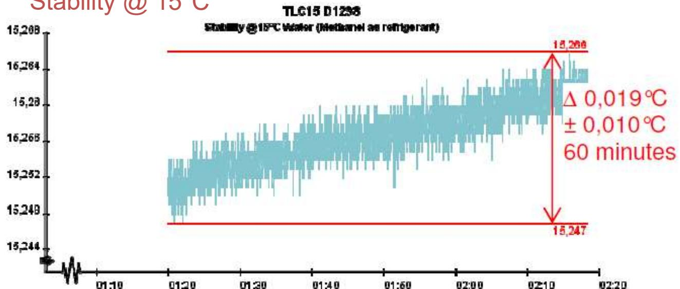
ASTM D1298 states that temperature should stay within  $\pm 0.25^\circ\text{C}$  of the test temperature. Our set-up easily meets this requirement.
