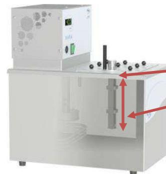
Liquid bath shall be fitted with suitable test tube holder to hold each test tube in a **vertical** position to a depth of about **100-mm** as measured from the bottom of the test tube to the bath surface.
