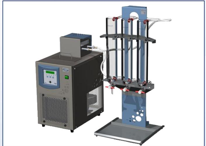
**Picture 4: ASTM D1298 Apparatus**
