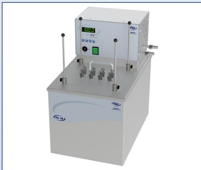
The TC16 can be used for immersing eight ASTM D565/D612 test tubes. The levelling platform (P/N 07T0210) keeps the test tubes above the 10 mL line and is required for operation. A special stainless steel cover (P/N 03T2314) with eight 16 Ø mm holes is required to suspend the test tubes in the bath.
