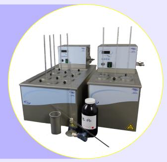
Position for 6 air wells with TC16 Position for 15 air wells with TC40 Stainless steel Bath drain Easy to operate Robust, well insulated
