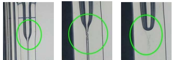
Prevent presence of fibres in the capillary
