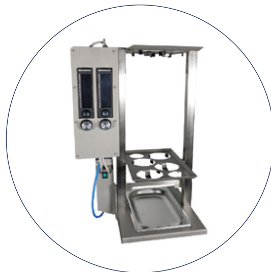
Rack with digital flowmeter
