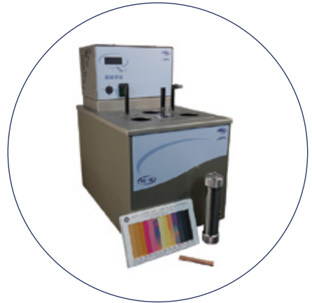
Copper Corrosion Bath
