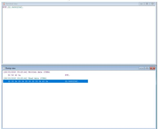
"Serial Port Monitor" is used to communicate and the window below explains all settings I think. In this case a RS232 to USB FTDI converter is used on port 4
